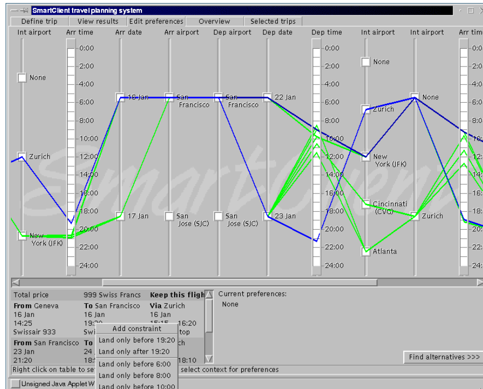
Figure 7. Edit preferences display allows the user to post preferences on any attribute of any displayed solution. Each solution is shown as a trace through the set of flight attributes. Constraints can be posted by using sliders and check boxes on the attributes.
